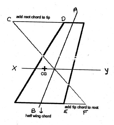
Draw a line between half the tip chord and half the root chord. (A 岛)
