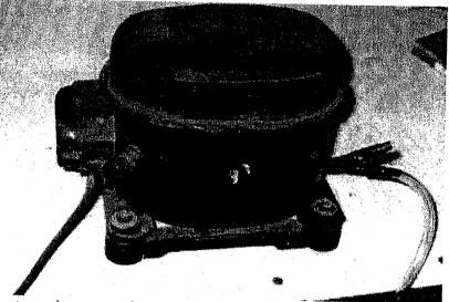
As you can see, it has two pipes, one for suck, and one for blow. With a bit of luck it will be as easily wireable as mine was. My pump will hold a vacuum. It doesn't leak when it is turned off. Some of my friends' pumps have a slight leak and you may want to make a valve up for stopping the backflow through the pump during the off phase.
